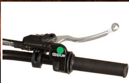
➡ New front brake master cylinder providing a better feel
