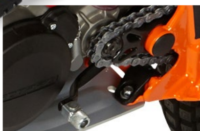
➡ Redesigned chain guide for improved frame protection
