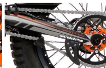
➡ New secondary drive (new sprocket and chain)
