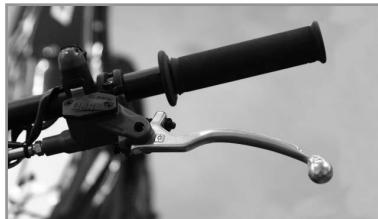
The clutch lever is on the left grip of the handlebar. To adjust the clutch lever's position, use the adjustment screw intended for this purpose (☞ p. 72).
