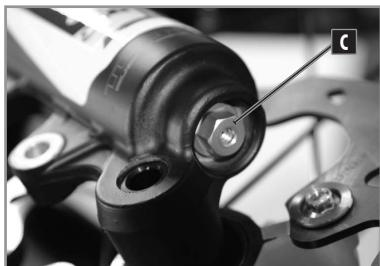
The Hydrostop ring determines how the shock absorber behaves in end position and resistance to the fork's impact.
