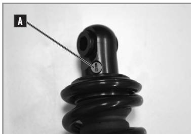
Adjust the shock absorber rebound with the adjustment screw **A**, located on top of the shock absorber.
