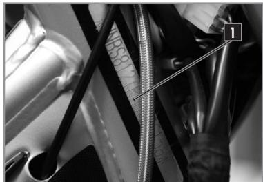
**1** The chassis's identification number is on the right side of the steering column.
