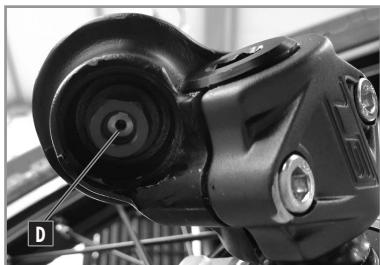
Adjusting shock absorption under compression influences the fork's behaviour while sagging.
