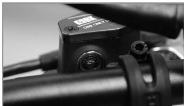
The front brake fluid tank is located next to the handle. It has a small viewer to check the fluid level.
