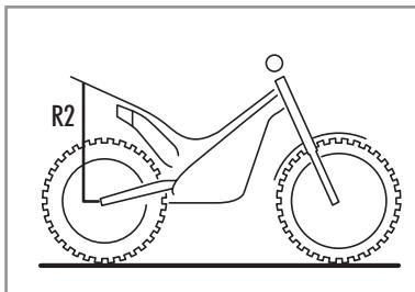
Determine the R2 no-load sag value of the shock absorber (☞ p. 88).
