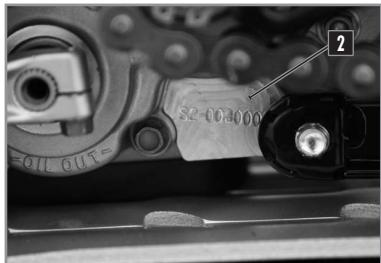
**2** The engine's identification number is on the left side of the chain guard, next to the gear selector.
