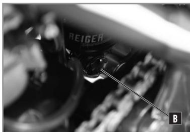
Adjust the shock absorber under compression with the knob at the bottom of the shock absorber.
