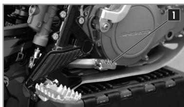
The rear brake pedal 1 is located in front of the right footrest.
