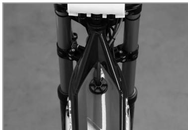
The fuel tank is designed for 2.2 litres.
