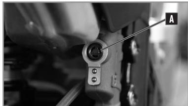
The brake fluid reservoir is located directly on the master cylinder.
