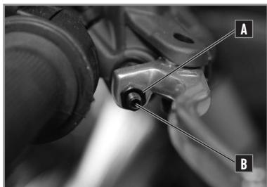
Adjust the tension of the front brake handle with the threaded rod **B**.
