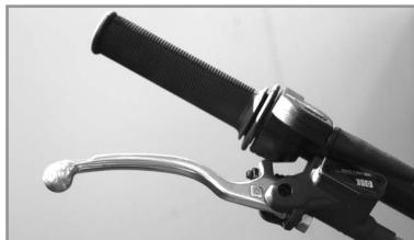
The front brake lever is located on the right grip of the handlebar.
