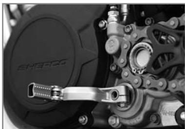
The gearbox consists of 5 positions, plus neutral.
