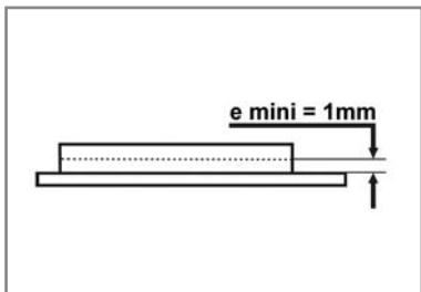
Wear on the thickness of pads occurs in the contact zone between the disc and the brake pads.
