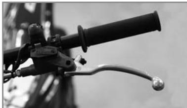
The clutch lever is on the left grip of the handlebar.
