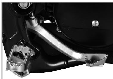
The brake pedal is positioned in front of the right footrest.
