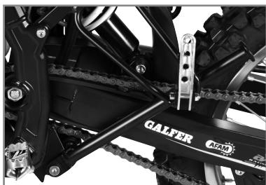
Lower the stand (left side) until it contacts the stop and then tilt the bike to the left until the base is in contact with the ground.
