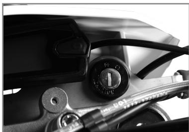
The bike has two keys (one is a spare) to be used for the ignition switch, to turn the engine on or off.
