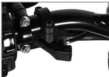
The choke lever is positioned on the left side handlebar. To operate the choke, press the lever.
