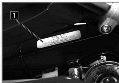
1 The chassis number is engraved on the right side of the steering column.
